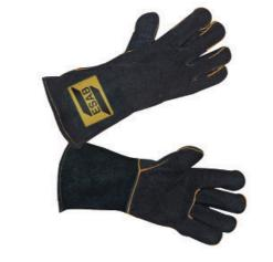
A welding glove made of black, strong cow-grain leather. High dexterity with KEVLAR stitching ensures that the glove can resist hard mechanical stress. Fully welted, CE approved. Cat. 2.
